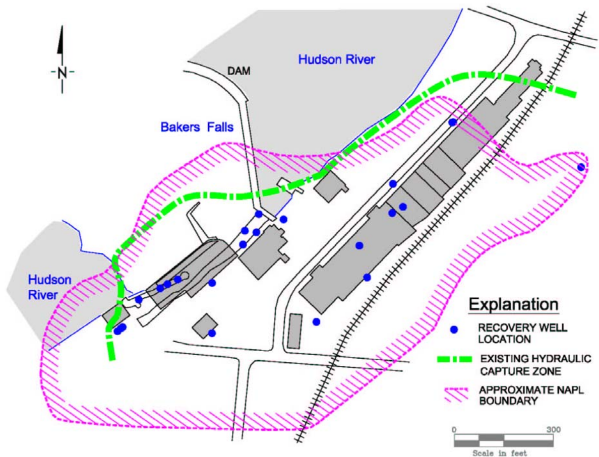
Figure 3. Site Contaminant Distribution Map
