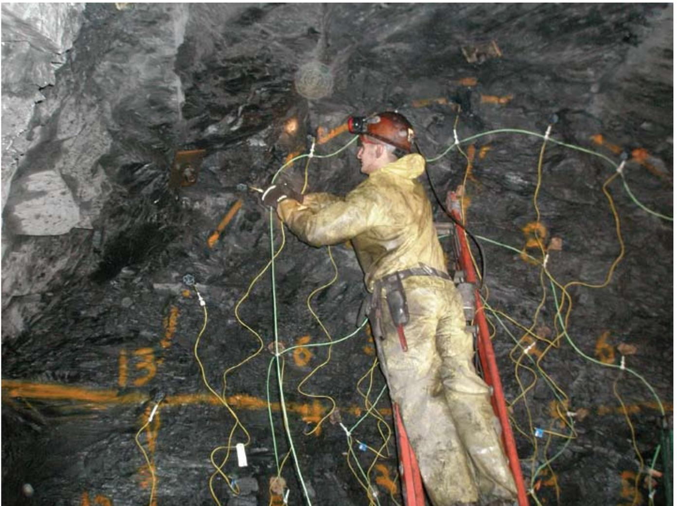
Figure 7. Tying up at heading.
