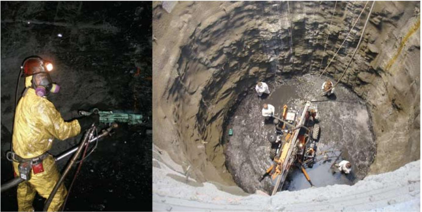
Figure 4. PPE during drilling operations at the TDCS.
