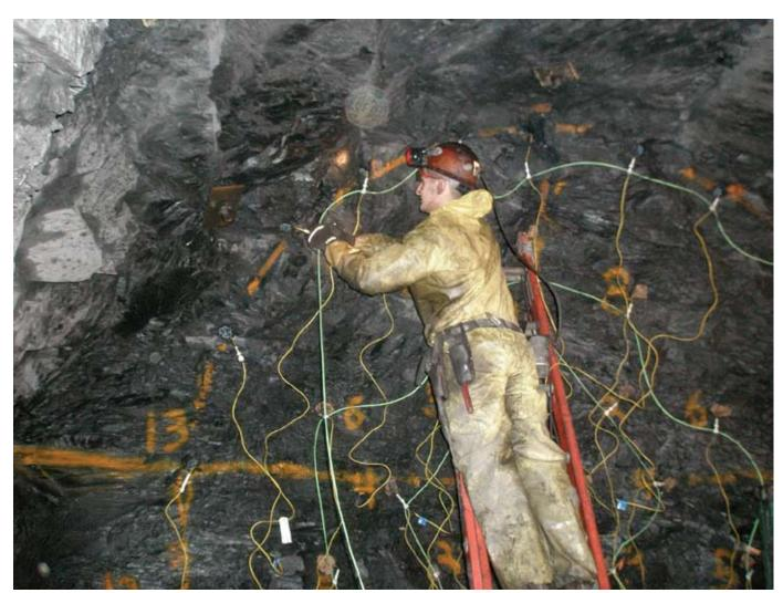
Figure 7. Tying up at heading.
