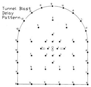
Figure 6. Typical tunnel blast design.
